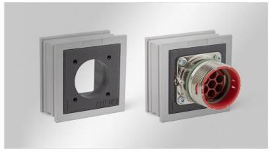
The grommet AT-FL is constructed on the basis of a large KT cable grommet. The polyamide body is moulded with elastomer. All square flanges with dimensions  $19.8 \times 19.8 \, \text{mm}$  (M23) can be integrated.
